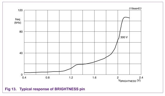
As can be seen in <u>Figure 13</u>, the frequency of the converter varies between a minimum frequency determined by the values of C7 and R8, and a maximum frequency determined by C7 and R9. The frequency is independent of converter input voltage and load fluctuations.
