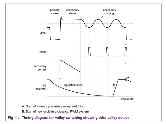
As can be seen from Equation 6, there is a trade-off between primary peak current, converter frequency and primary inductance. The primary peak current helps determine switching losses, as does the switching frequency. The ratio of the primary inductance to peak current determines the core size. Common frequencies are 50 kHz (in EMC-susceptible environments) and 100 kHz.
