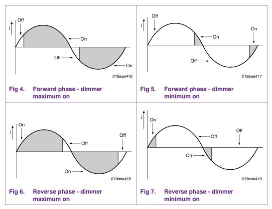
Two switching methods can be distinguished: triac dimming and transistor dimming. Triac switching is always used with forward phase dimmers. Transistor switching can be used with forward and reverse phase dimmers. Transistor dimmers have the advantage of being able to switch capacitive loads, but most existing dimmers are still triac based.
